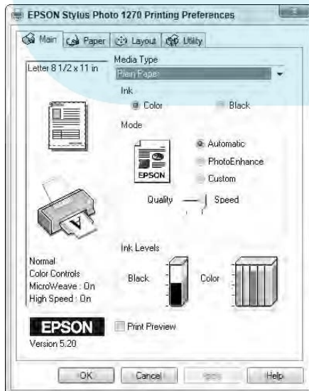
Figure 4-7: Some printers let you check the cartridge's ink level directly from Windows.
